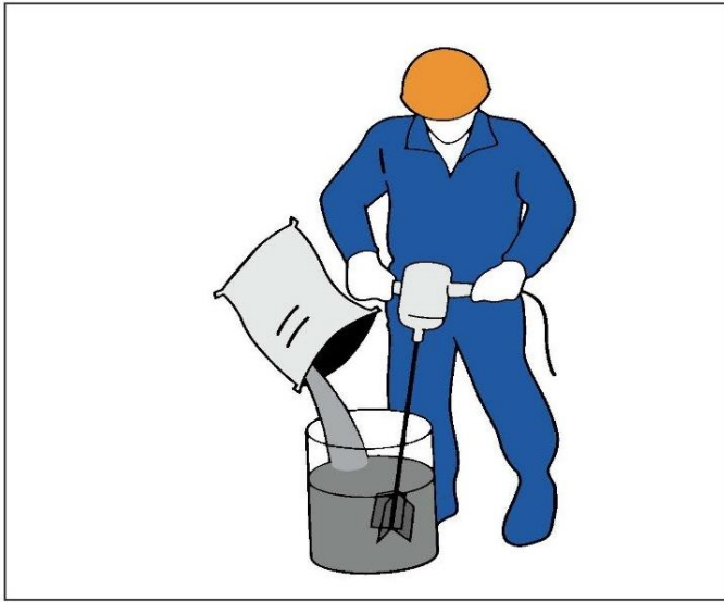
Figure 1: Mixing the grout with a birdcage paddle on the mixer
